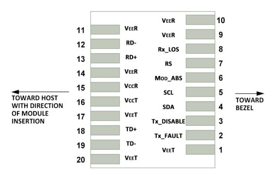
Host PCB SFP Pad Assignment Top View
